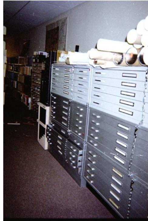
Photo 3: Library map cases constrained using Schuster chains
